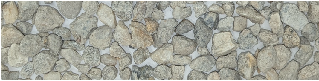
Fig. 1 Coarse recycled concrete aggregate 4/16.
