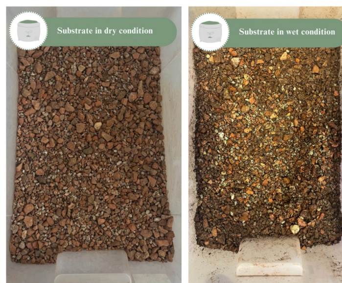
Fig. 3 Roof substrate in dry and wet conditions.
