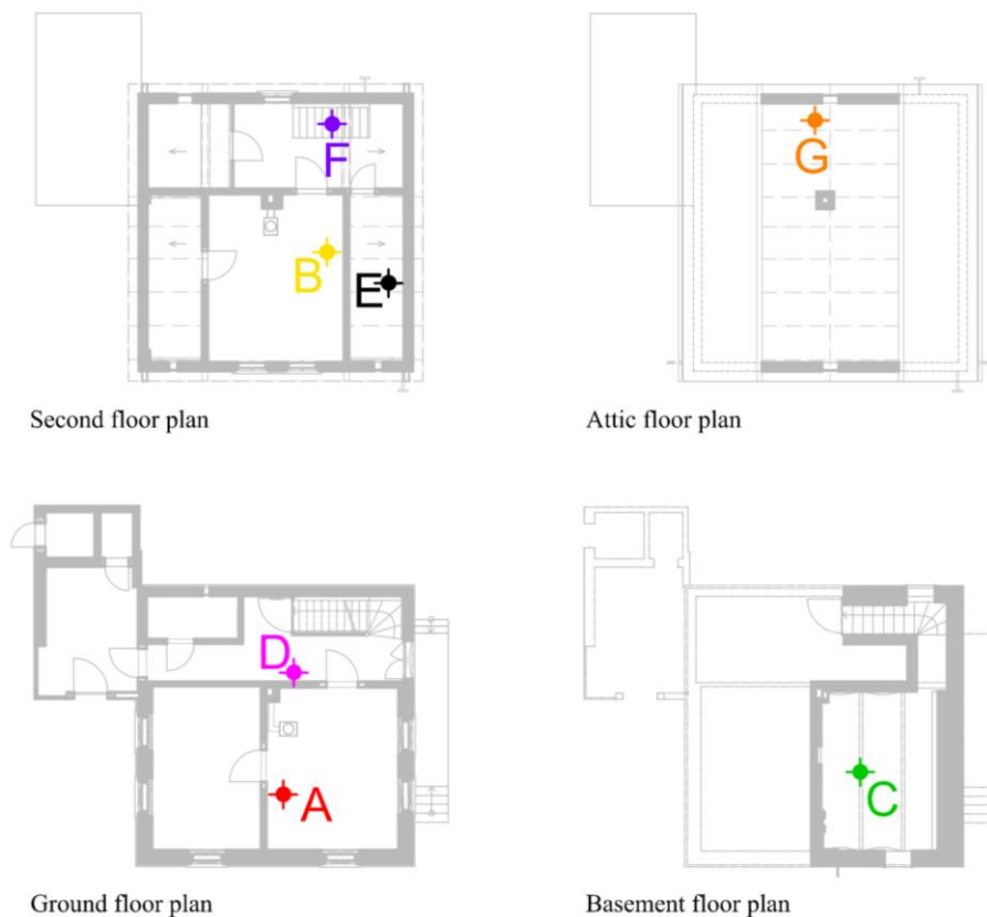
Fig. 2 The plans of the case study house with positions of dataloggers. Dataloggers U3430 were used in the living areas (A – living room, B – bedroom). Dataloggers U3120 were used in unoccupied rooms (C – basement, D – corridor on the ground floor, E – chamber under the roof, F – corridor on the second floor, G – attic, H – outside).
