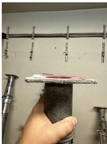
Fig. 3 Bent steel plate.
