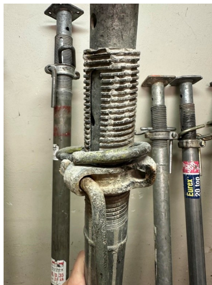
Fig. 2 Broken thread on the support.
