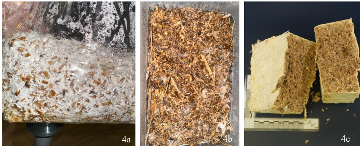
Fig. 4 Growth Process of Sample 1(Heads); 4a- Mixture after mycelium growth, prior to moulding; 4b- One day after moulding - beginning of growth process; 4c- Sample after drying process.
