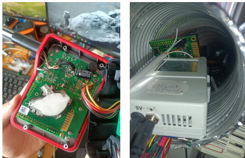
Fig. 2 Left: CL11 disassembly. Right: placement in the duct.
