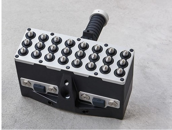
Fig. 3 Matrix probe of Pundit 250 Array.
