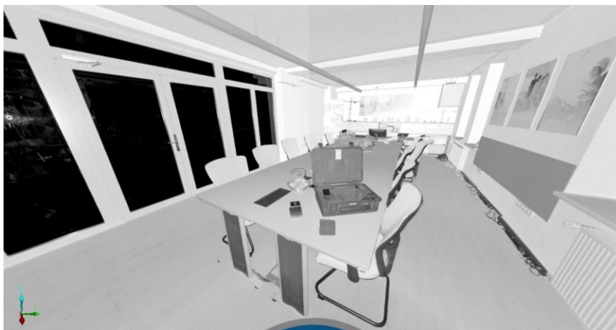
Fig. 3 Point cloud created by terrestrial scanner.
