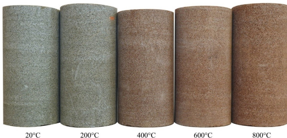
Fig. 2 The fired glauconitic sandstone specimens used for the CTT_{II} s ( D = 38.1 mm, L/D \sim 2.0 ).
