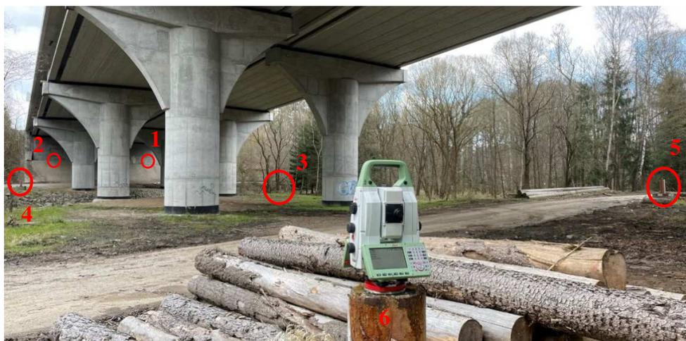
Fig. 2 Leica Nova TS60 at point 6.
