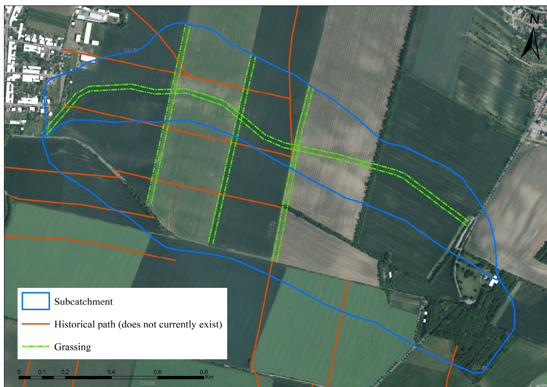
Fig. 9 Variants of measures (var. 0: current state, var. 1: just considered historical paths, var. 2: grassing of thalweg and three grassing strips).
