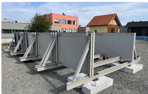
Fig. 1 Fully composite modular footbridge with a span of 8.0 meters.
