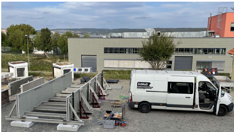
Fig. 4 View of the loading test with the applied force in the horizontal direction.
