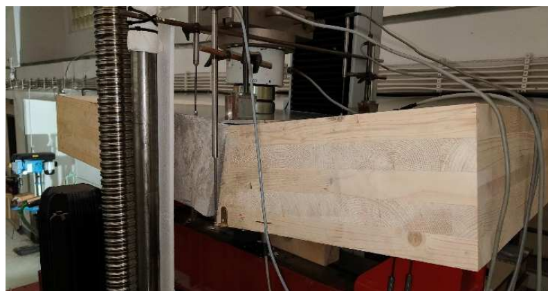
Fig. 30 Failure of specimen A.
