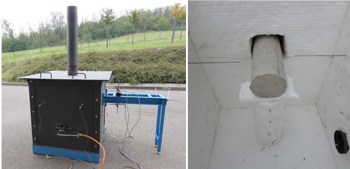
Fig. 4 Test setup for reinforcement fire conditions.
