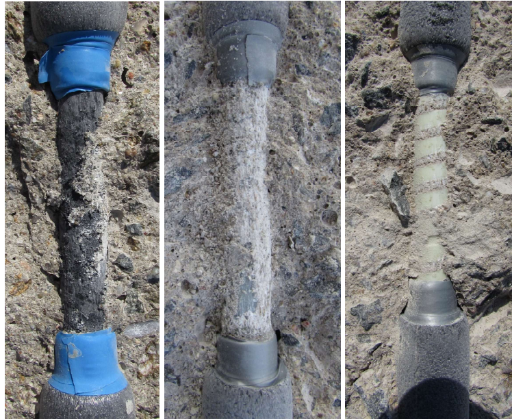
Fig. 8 Typical failure of the reinforcement in pull-out tests under normal conditions a) RockBar "BN", b) ReBar "PN", c) ComBAR "CN" (left to right).
