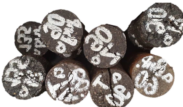
Fig. 2 Test specimens after indirect tensile strength test.
