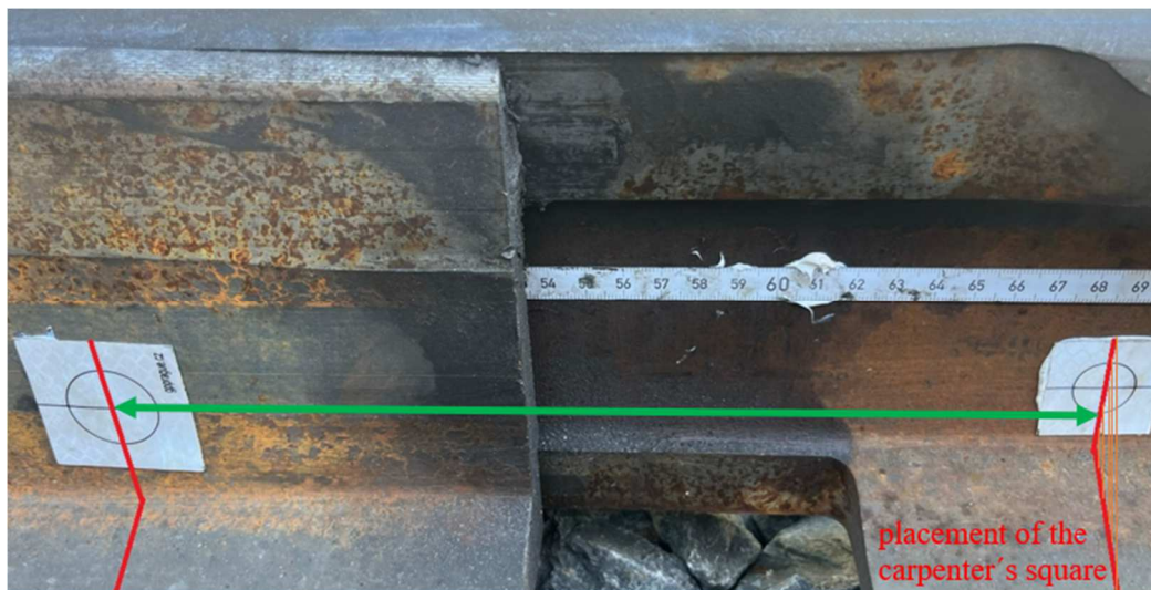
Fig. 4 Marking of the second measurement method of the mutual position of the tongue and the knee rail.
