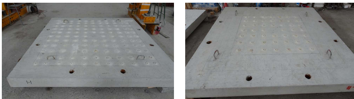
Fig. 3 Drilling holes in specimen S_{4d} (left) and S_{3d} (right).
