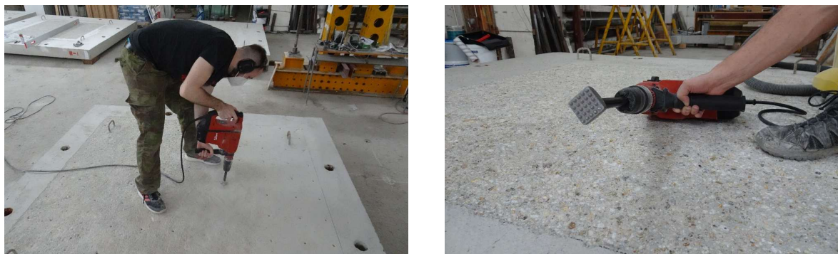
Fig. 4 Roughening the surface of the reference slab specimen.
