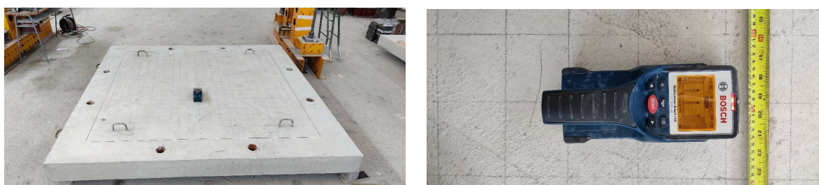
Fig. 2 Mapping of existing rebar by a magnetic scanner.
