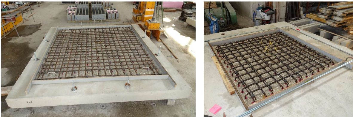
Fig. 6 Reinforcement of specimens S_{4d,SD} (left) and S_{3d,SDR} (right).
