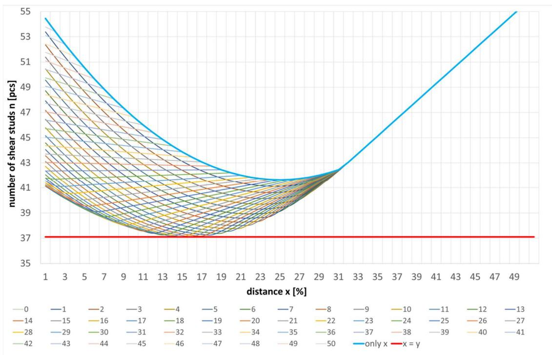
Fig. 7 Graph of the dependence of the number of shear studs on the percentage increase of the length of sections  $x$  for different lengths of section  $y$  (its percentage increase), including the influence of design principles. It includes the plotted results for the case with only two shear studs spacings (with only an  $x$ -section) and the case of distribution according to the configuration in Fig. 3.
