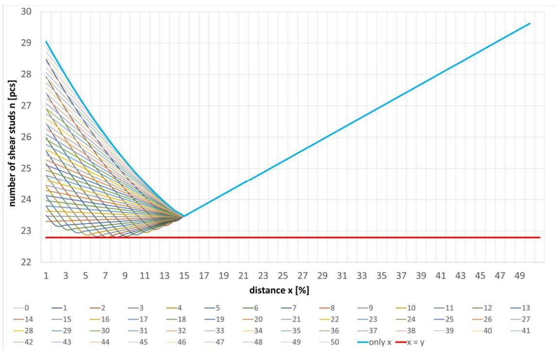
Fig. 8 Graph of the dependence of the number of shear studs on the percentage increase of the length of sections  $x$  for different lengths of section  $y$  (its percentage increase), including the influence of design principles. This is the case where the limit imposed by the design principles comes into effect before 1/6 of the beam span.
