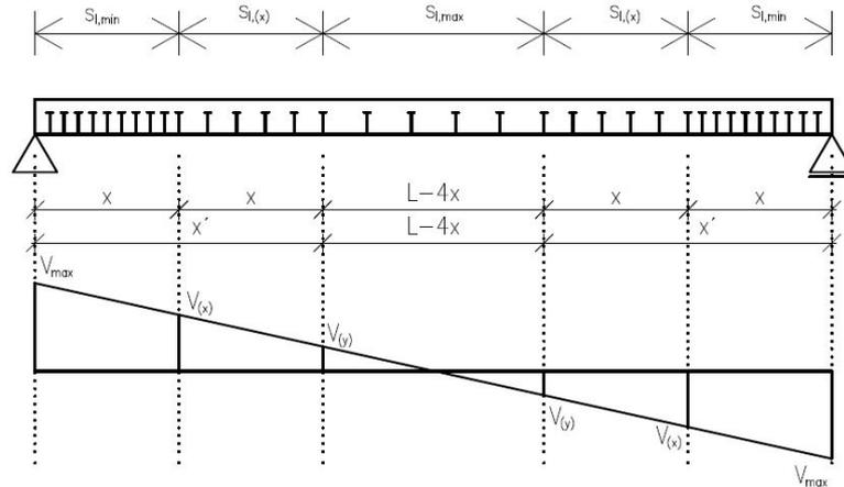
Fig. 3 Scheme of the shear stud layout configuration, where the maximum allowable stud spacing is applied along the entire length to which the limit of the design principles is relevant and the remaining edge parts are divided into two equal sections.
