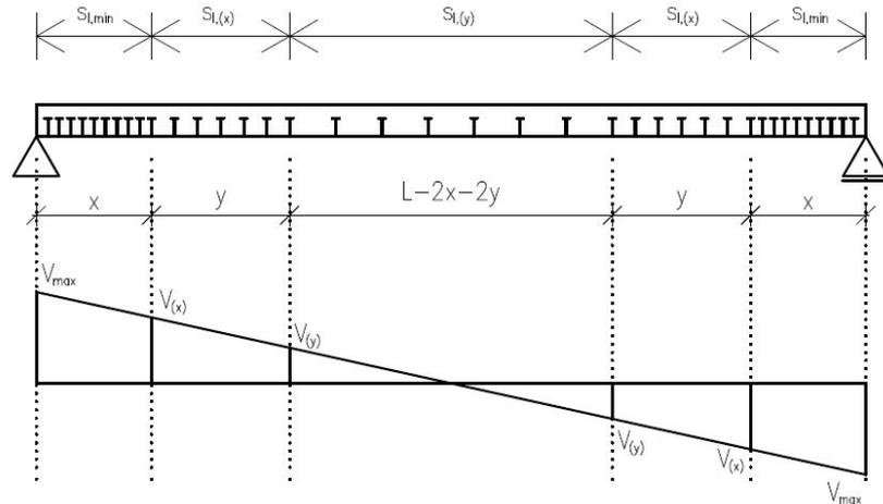
Fig. 1 Diagram of the shear stud distribution on a beam using three spacing sizes where the spacing change is at distance  $x$  and  $y$ .
