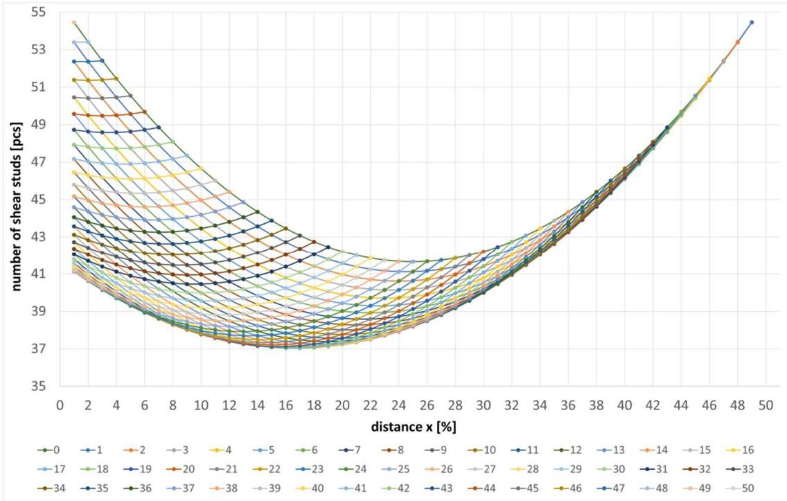
Fig. 5 Graph of the dependence of the number of shear studs on the percentage increase in the length of sections  $x$  for different lengths of section  $y$  (its percentage increase), for the ideal condition with no limitations from the design principles.
