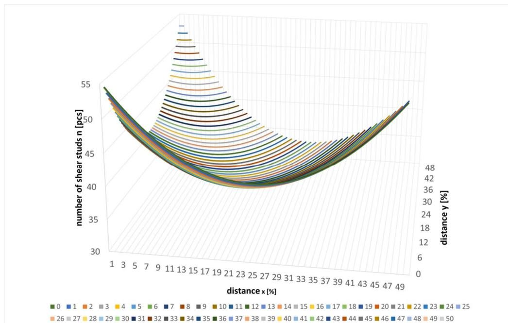
Fig. 4 Spatial graph of the dependence of the number of used shear studs on the length of the  $x$  and  $y$  sections in which the change of spacing was made. The graph is for the case without the limitations of the design principles.
