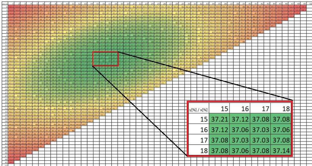
Fig. 6 A colour scale representing the amount of shear studs for percentage values of the lengths of the  $x$  and  $y$  sections from 1 to 49 for ideal conditions without the influence of limitations from the design principles, where green indicates the minimum number of studs and red the maximum.
