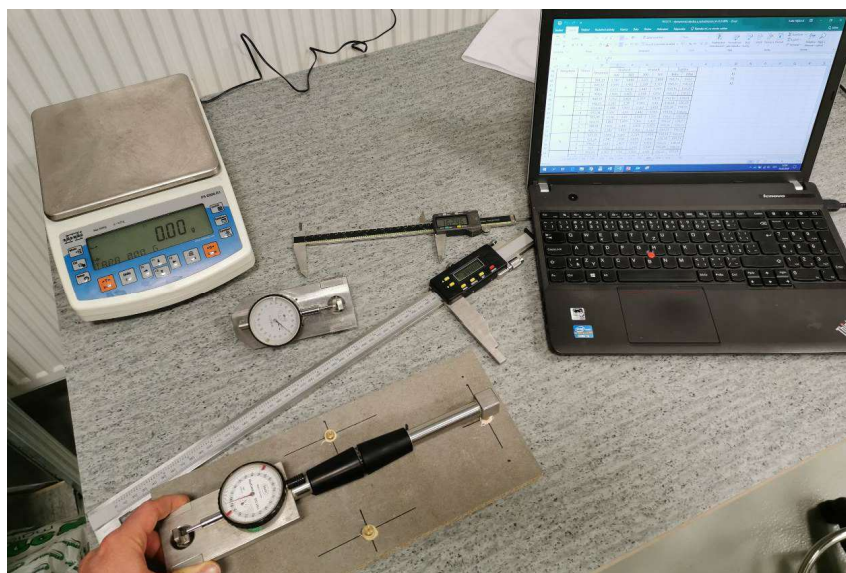
Fig. 5 Determination of the mass and dimensions of test specimens during the absorption of air humidity (specimen removed from climate chamber).
