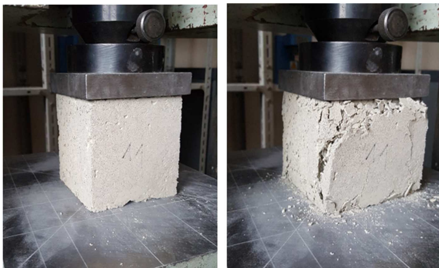
Fig. 3 Compressive strength measurement.
