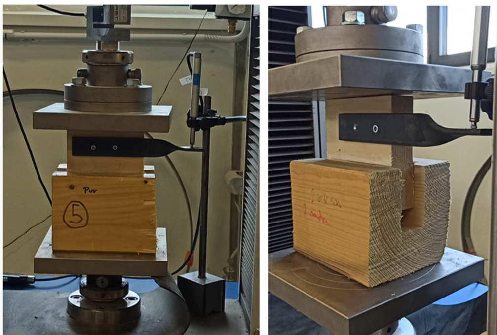
Fig. 2 Specimens in the test equipment TIRA test 2850 S.
