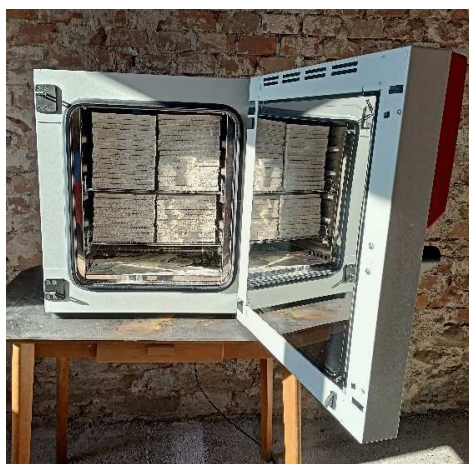
Fig. 2 Cycling: storage of test of a real joint in a drying oven.
