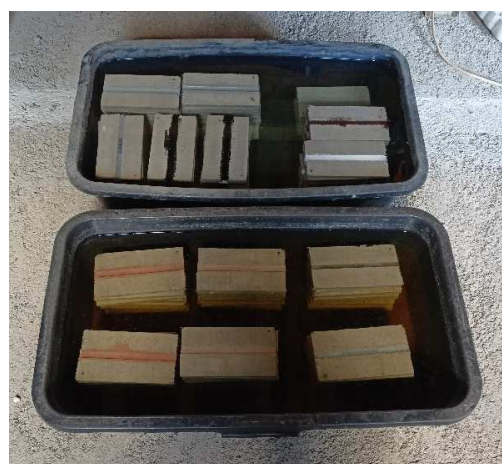
Fig. 3 Cycling: storage of test of a real joint in water.
