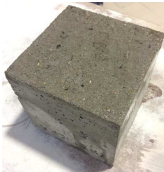
Fig. 2 Test sample of concrete with road cement after the durability test of the cement concrete surface against the action of water and chemical deicing agents.
