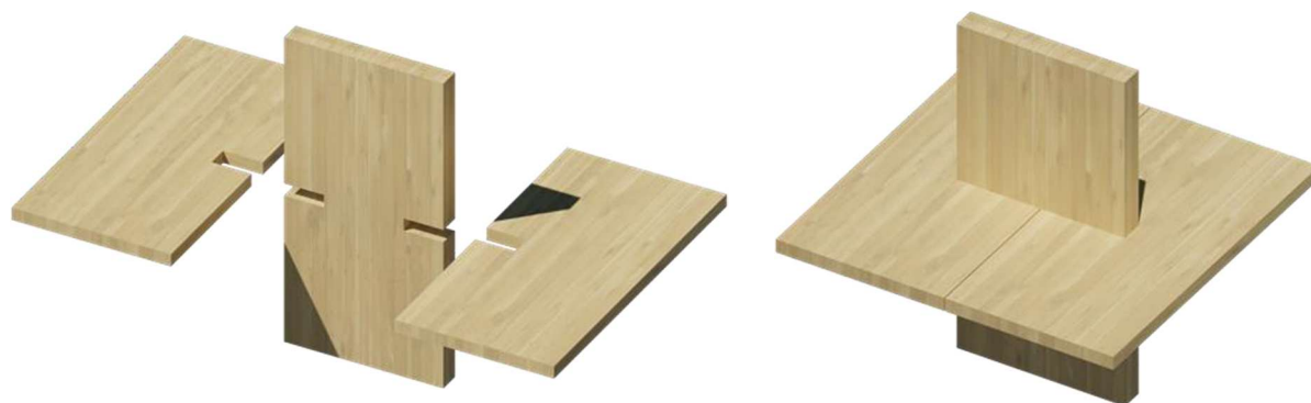
Fig. 4 Diagram of the jointing of basic units.
