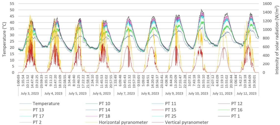
Fig. 8 Graph of the dependence of the air temperature in the narrow cavity on the outside air temperature and the intensity of solar radiation from 3<sup>rd</sup> to 12<sup>th</sup> July.
