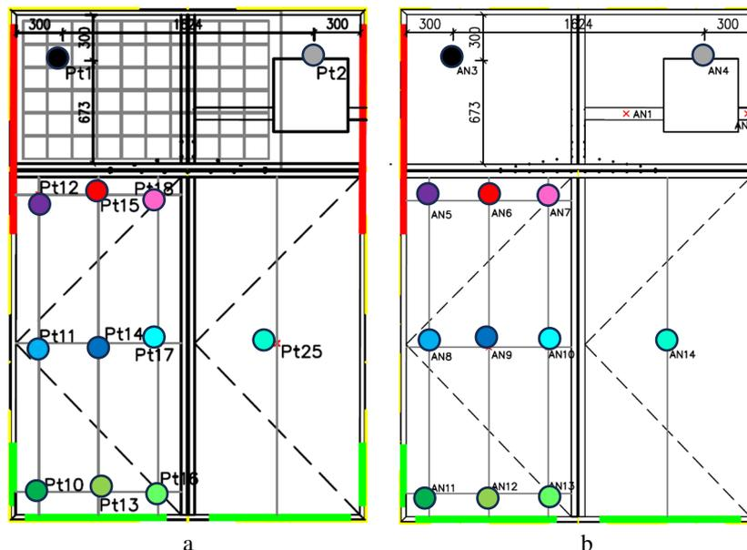
Fig. 5 Sensors used for summer mode analysis. Layout of Pt 100 sensors (PT) and anemometers (AN) in the innovative DSF (view from interior). The green lines represent inlets and the red lines denote outlets.
