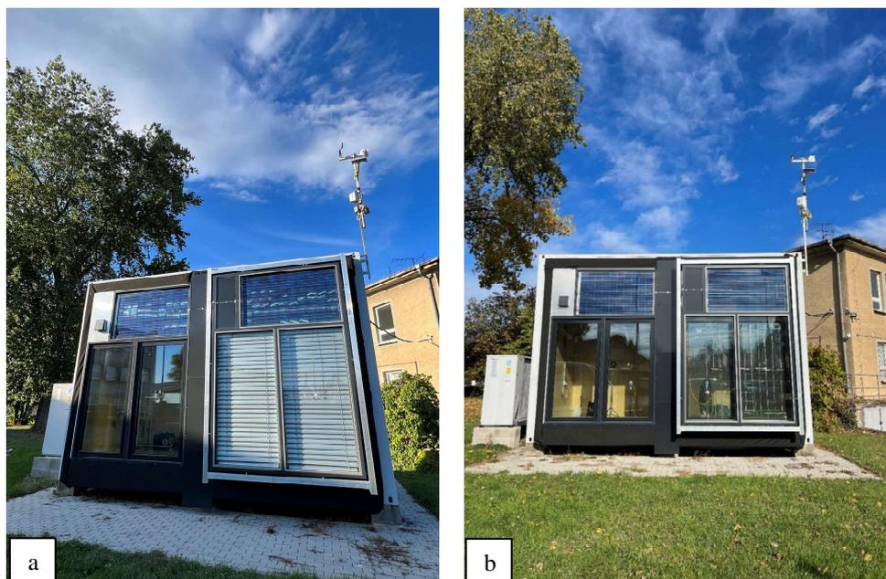
Fig. 2 A view of the facades installed at the Twin Rooms experimental facility (a simple facade installed on the left side, with the same geometric and physical parameters as the inner wall of the double skin facade and an innovative double skin transparent facade installed on the right side), a – the facades in the summer period, b – the facades in the winter period.
