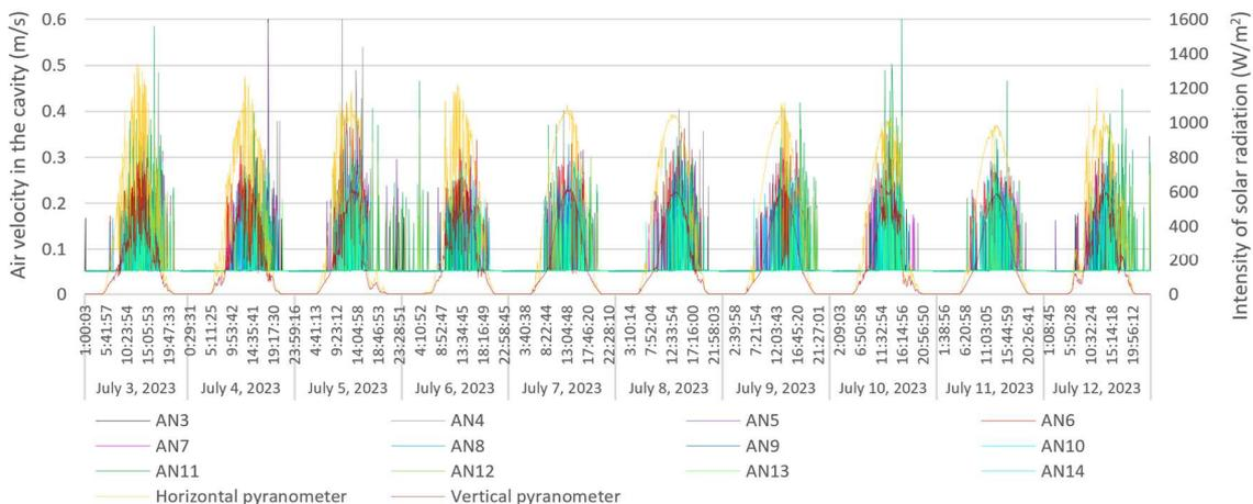
Fig. 7 Graph of the dependence of the air flow rate in the narrow cavity on the intensity of solar radiation from 3<sup>rd</sup> to 12<sup>th</sup> July.
