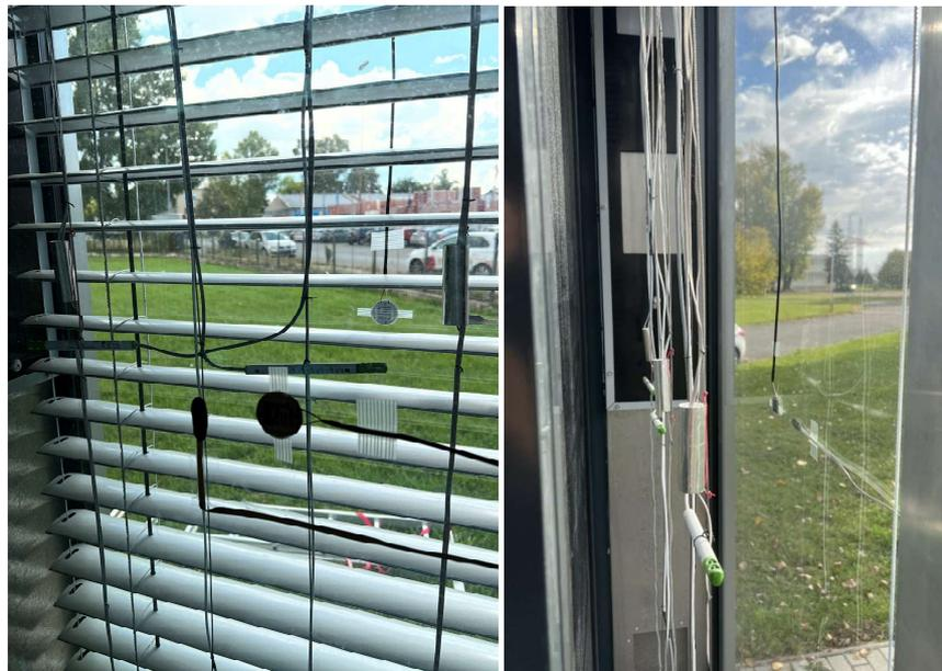
Fig. 3 Measuring equipment installed in the double skin transparent facade with a narrow cavity (280 mm wide): anemometers, Pt 100 sensors and heat flux sensors (equipment used for analysing DSF values in this paper).
