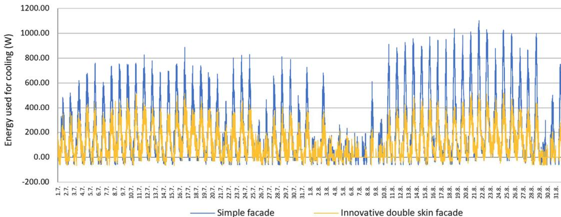
Fig. 9 Graph showing the cooling performance of the simple facade and innovative double skin facade from 1<sup>st</sup> July to 31<sup>st</sup> August 2023.
