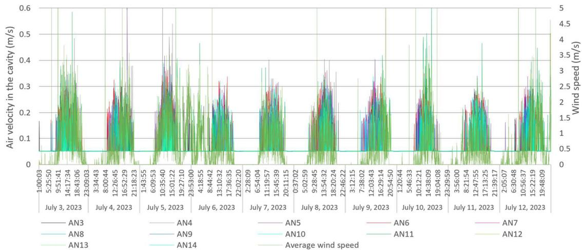
Fig. 6 Graph of the dependence of the air flow rate in the narrow cavity on the wind speed from 3<sup>rd</sup> to 12<sup>th</sup> July.
