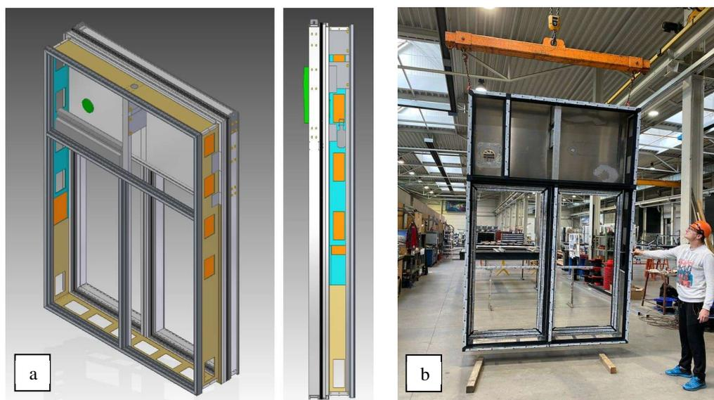
Fig. 1 Model of the innovative facade, a – 3D model, b – prototype during production.
