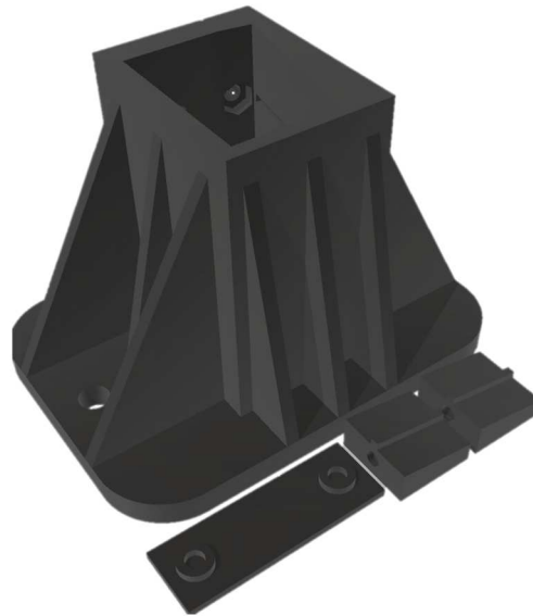
Fig. 2 3D model of the fixture used to hold the specimen for the shear test.
