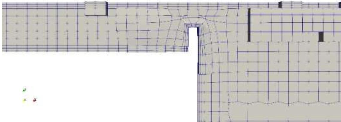
Fig. 3 Mesh of 300 thousand cells, detailed inlet (CfMesh).
