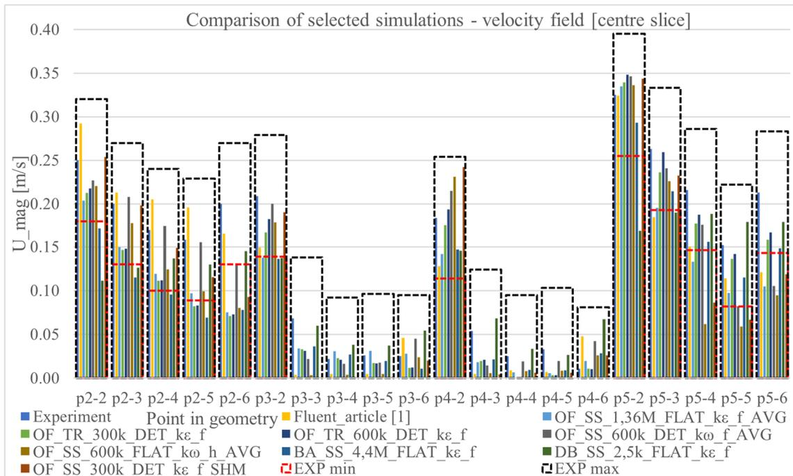
Fig. 6 Velocity field results comparison.
