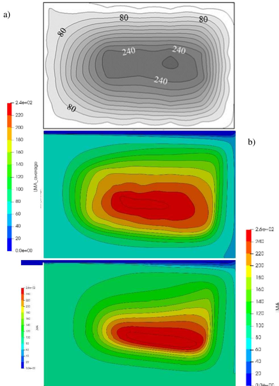
Fig. 5 LMA: a) from article [2]; b) averaging – 300 thousand cells; c) averaging – 1,200 thousand cells.
