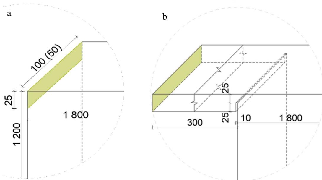
Fig. 4 Inlet types: a) flat inlet b) detailed inlet.
