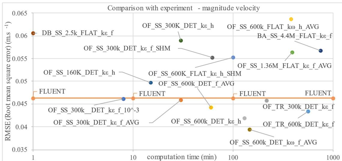
Fig. 8 RMSE for velocity – comparison with experiment.
