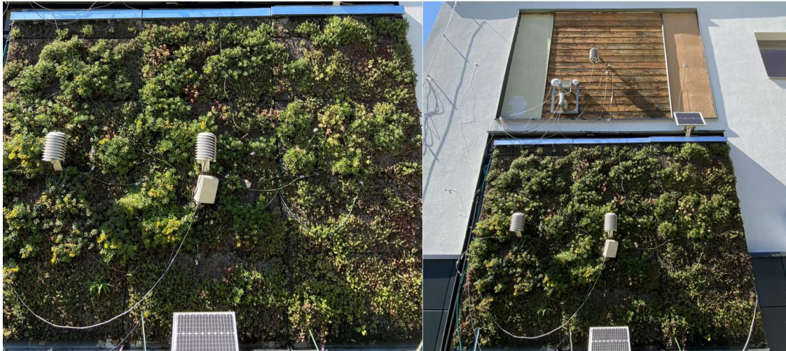
Fig. 3 View of the vegetated façade sample (left) and location in relation to the timber columned structure sample (right).
