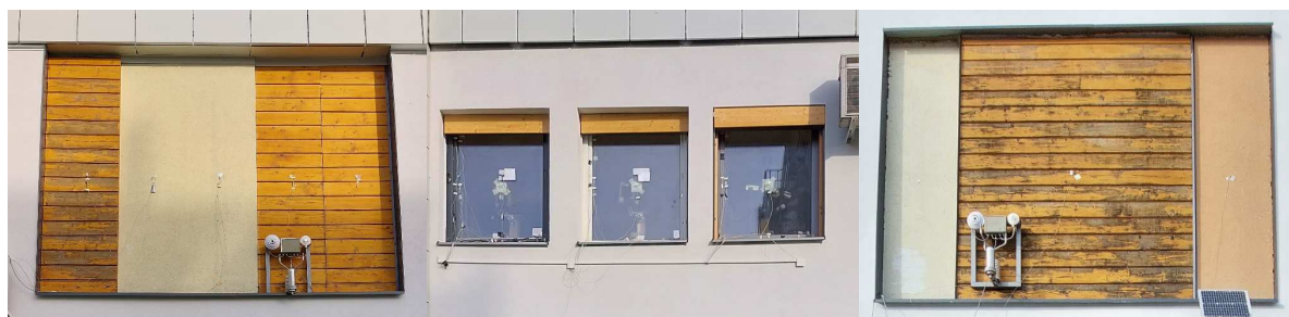
Fig. 2 View of the timber post and window samples from the exterior side (south sample on the left, window structures on the south side in the middle, east sample on the right).
