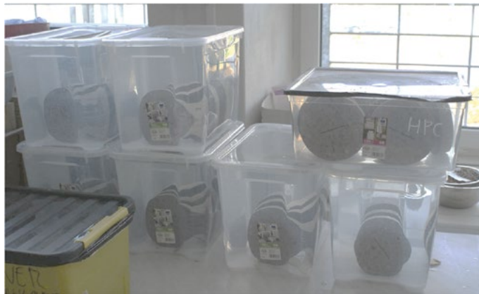
Fig. 1 Prepared BD and BDCN specimens stored in plastic containers filled with water and chloride solution in a laboratory room with a constant room temperature.
